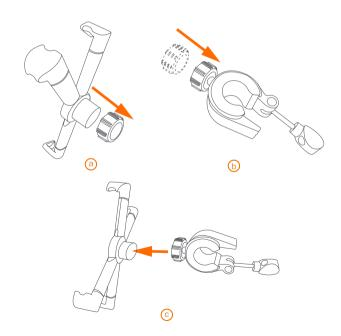
2 Attach the phone holder to the handlebar and adjust it to the proper position.
