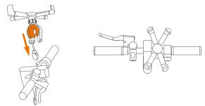
3 Rotate hand screw to the slot of buckle and tighten hand screw, adjust the phone holder to the appropriate angle, and tighten adjustment nut.
